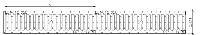
GALVANISED STEEL GRATING COVER FOR LOAD CLASS ACCORDING TO EN 1433
